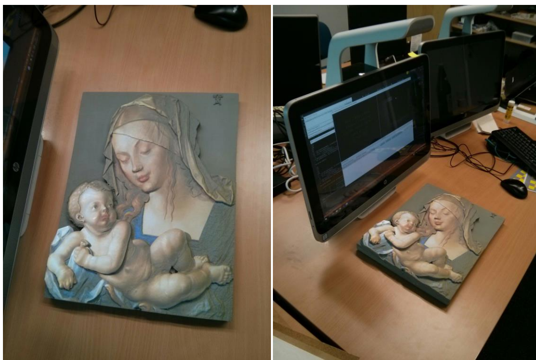
Figure 41: Projection of the original coloured image onto a tactile relief. Note that the projection quite exactly matches the relief, thanks to our new calibration method.
