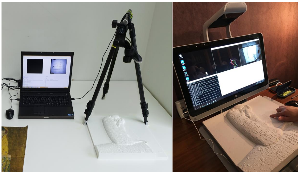
Figure 33: Comparison of old and new setup, © ARCHES project team. From left to right: (a) previous prototype setup using a tripod mounted RealSense F200 depth camera. (b) User testing the new setup with HP Sprout, making a pointing gesture. Depth camera and projector are integrated in the top part of the device. The relief is simply placed on the table.
